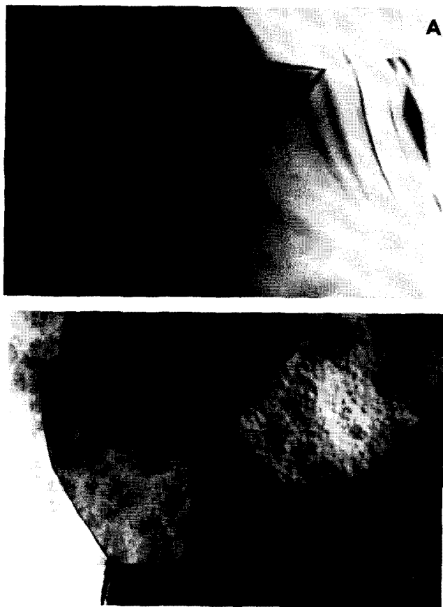
Fig. 10. Bright-field (BF) TEM micrographs of mixed oxide pellet sintered at 1260°C for 2 h indicating (a) crystalline second phase at grain junction (S) and (b) grain structure and clean grain boundaries.
