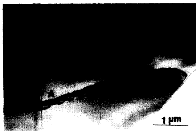
Fig. 13. Typical planar defects observed in PMN pyrochlore produced from both mixed oxide and partial oxalate methods (1260°C, 2 h).
